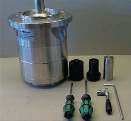
1. Unscrew the 4 mounting screws and remove the seal SAE flange. **Do not yet unscrew the 2 lower screws.**
