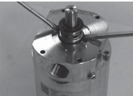
3. Ensure that no dirt has entered into the pump. **IMPORTANT: If loose particles are observed, the pump must be dismantled and thoroughly cleaned with clean (filtered) water.**
