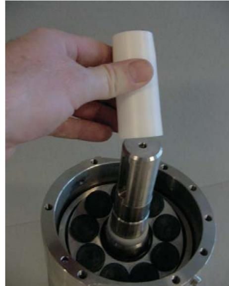
5. Thoroughly wet the torpedo, shaft and replacement shaft seal with plenty of soap. **Do not use silicone grease.**
