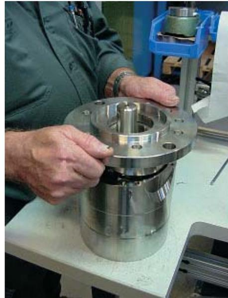
11. Screw the 4 screws into the flange and the housing. **To prevent cold welding, lubricate the threads on the 4 screws with grease**, screw them into the pump and tighten by hand. Use Molykote® D paste from Dow Corning or Klüber UH1 84-201 from Klüber lubrication.
