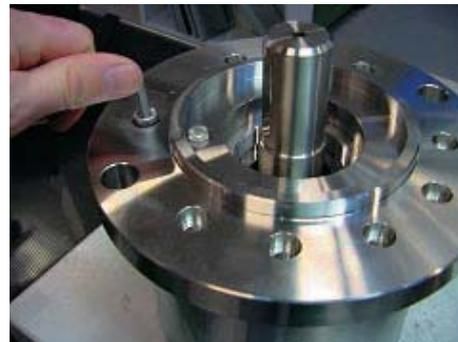
12. Tighten the 4 flange screws to a torque of  $8 \pm 1$  Nm using the tool provided.
