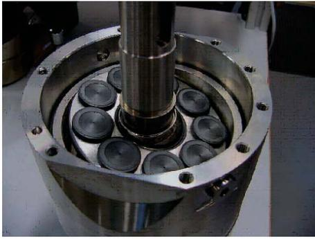
8. Use the plastic assembly tool provided, **large diameter pointing downwards**, to press the seal home against the shoulder of the spacer.
