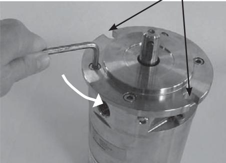
2. Wet the shaft and shaft seal with clean (filtered) soap-water. Gently lever the shaft seal assembly free using 2 screwdrivers.
