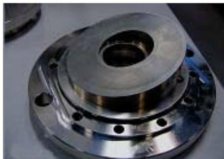
10. Wet the new ceramic ring with clean (filtered) soap-water and fit it on the flange using the plastic tool provided. Ensure that the rubber seal is positioned against the shoulder of the flange.
