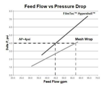
Pressure Drop versus Feed Flow for Mesh wrap and FilmTec™ Hypershell™ 8038 elements. FilmTec™ Hypershell™ has less exterior bypassing and requires approximately 30% less flow than mesh wrap for an equivalent pressure drop.
