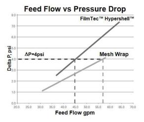
Pressure Drop versus Feed Flow for Mesh wrap and FilmTec<sup>™</sup> Hypershell<sup>™</sup> 8038 Elements. FilmTec<sup>™</sup> Hypershell<sup>™</sup> has less exterior bypassing and requires approximately 30% less flow than mesh wrap for an equivalent pressure drop.
