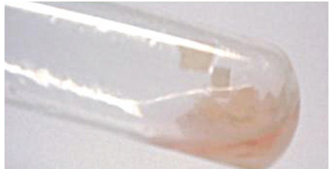
Membrane oxidation damage
