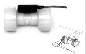
Engineered specifically for small pipe diameter applications, the Signet 2100 Turbine Flow Sensor provides accurate readings in two flow ranges: 0.3 to 3.8 lpm and 3 to 38 lpm (0.1 to 1 gpm and 0.8 to 10 gpm).
